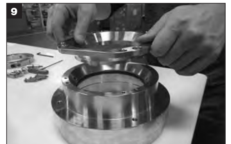
Invert gland assembly. Remove shoulder screws and discard. Lift pusher from gland assembly.
