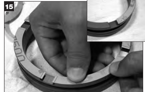
Place the rotary seal face on a dry clean cloth face side down to avoid scratching or damaging the face. Peel the adhesive backing from the rotary cushions. Align scored edges with edges of slots and press to ensure adhesion to that surface.
