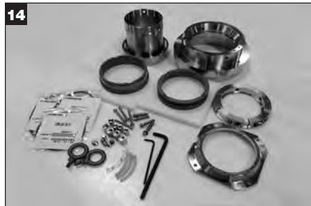
Remove spare parts kit components from packaging and place on a clean work surface. NOTE: Leave the two largest O-Rings packaged for size identification.
