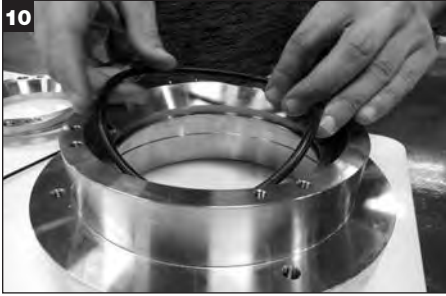
Remove O-Ring from gland inside diameter and discard.
