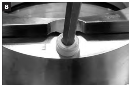
Remove old pipe plug if it is still installed and discard.
