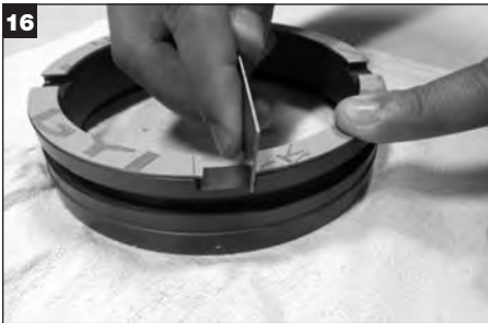
Fold the cushion tabs into the slots and press them in against the drive slot edge with a straight edged tool or ruler.
