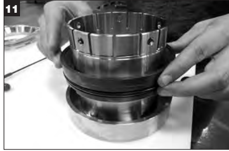
Remove rotary seal ring from sleeve and discard.
