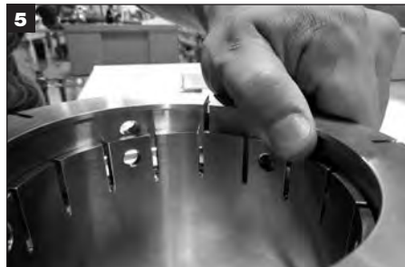
Remove lock ring from sleeve.
