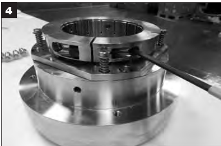
Remove dog point set screws and TORX screw from lock ring and discard.
