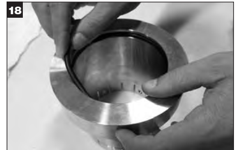
Apply a thin film of grease to the shaft O-Ring and install in the sleeve inside diameter groove.
