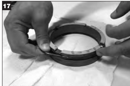
Apply a thin film of grease to the rotary O-Ring and install in the rotary seal face outside diameter groove
