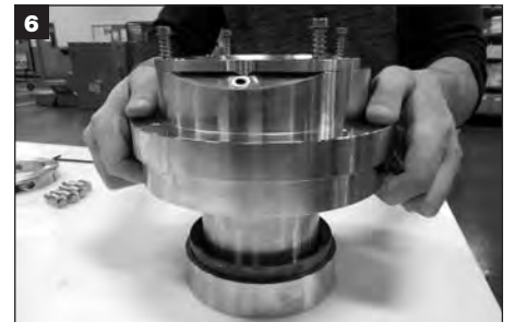
Separate gland assembly from sleeve assembly.
