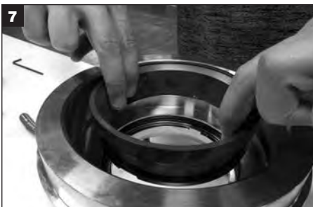
Invert gland assembly and remove stationary seal ring and discard.
