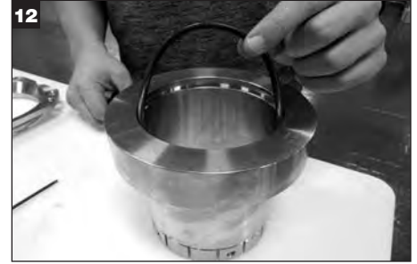
Remove shaft O-Ring from sleeve inside diameter and discard.
